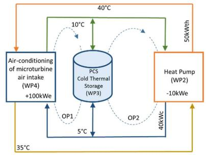
OP1: Air intake cooling (HP is off) – Max net power output OP2: Air intake heating (HP is on) – Min net power outut
